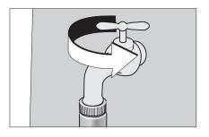
**Step 4**Connect garden hose to the cold water source and turn water on completely.
